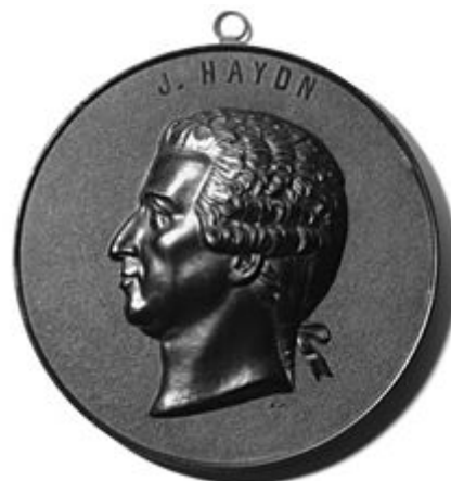
A decorative medal made in France in the early 20th century moulded from shellac compound, the same used for phonograph records of the period
